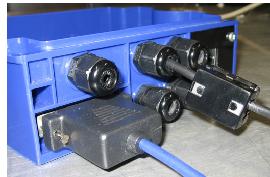
Figure 5 – Ferrite Installation Example
