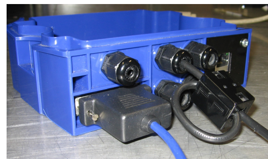
Figure 6 – Ferrite Installation Example
